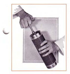
The bobbin is of metal, the part carrying the paper being in two sections, with a narrow slot between. This slot is arranged to close by screw motion, the closing action both stretching the paper and holding it perfectly taut. This type of bobbin is available  $3\frac{1}{2}$ in (90mm) or 5in (125mm) diameter. Alternative metal type can be supplied  $2\frac{1}{4}$ in (55mm) or  $2\frac{3}{4}$ in (70mm) diameter.
